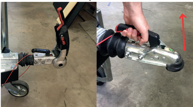
Figure 9; raise the stabilizer to the highest setting.
