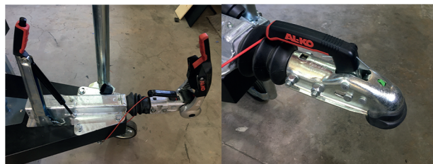
Figure 6.1; AL-KO coupling and stabilizer.
